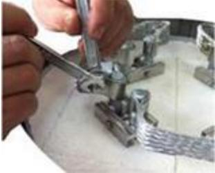
**2. Unscrew the electrical contacts** of heating elements with a wrench (*supplied as an accessory*).
