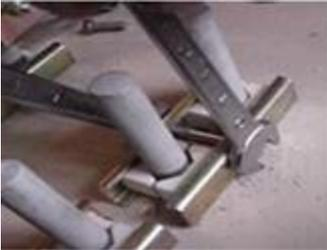
**4. Unscrew the support elements** of heating element with a wrench (*supplied as an accessory*).
