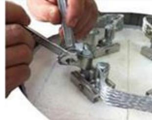
**2. Unscrew the electrical contacts** of heating elements with a wrench (*supplied as an accessory*).
